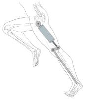
Highly reliable The non-contact transmission has very low noise, no wear, no friction and no risk of jamming. This also removes the need for lubrication from all but the external bearing races holding the actuator rod.
